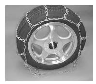
Drape the chain over the tire, so that one cross chain is postioned at the point where the tire meets the ground. Again make sure the cross chain hooks are facing upward. Hooks that face down (towards the tire) will cause damage to the tire.
