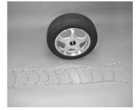
Park vehicle on firm level ground, and turn off the engine. Set the parking brake. Unroll the chains and lay them out flat on the ground making sure there are no twists or tangles. Make sure the smooth side of the cross chain hooks are towards the tire.
