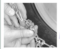
Reach behind the tire and engage the inside connector on the 2nd or 3rd link. See the illustration on the next page for a detailed look at this connection.
