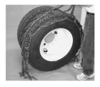
Park vehicle on firm level ground, and turn off the engine. Set the parking brake. Lay the chains out flat on the ground, making sure there are no twists or tangles. Make sure the cross chain hooks are facing upward.
