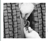
Reach behind the tire and engage the inside connector making sure it is as tight as possible. Then connect the center (between the duals) fastener in the same manner. See the illustration on the next page for a detailed look at this connection.
