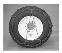
Security Chain Co. recommends that chain tighteners (sometimes known as chain spreaders) be used to take up additional slack. To make this simpler, attach the first hook at the "11 o'clock" position, the next at the "5 o'clock" postion and so forth. The open side of the hooks must face away from the tire. No further adjustment should be necessary.
