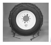
Drape the chain over the tire, so that one cross chain is postioned at the point where the tire meets the ground. Again make sure the cross chain hooks are facing upward. Hooks that face down (towards the tire) will cause damage to the tire.
