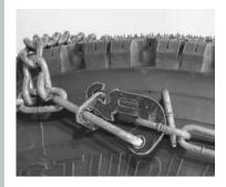
Next fasten the outside fastener, again making sure it is as tight as possible. Drive a short distance and retighten all fasteners. For best results, make sure all connections are equal and as tight as possible.
