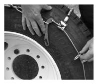
Fasten the outside connector by passing the long lever through one of the chain links, folding it back in the opposite direction and securing the "keeper" link on the end of the lever. If care is taken to make this connection as tight as possible, it may not be necessary to retighten after driving. If you find that the inside fastener also has to be adjusted to assure a snug fit, you should do it before fastening the outer fastener.
