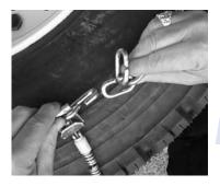
Connect the "speed hook" on the inside of the tire (the side away from you). As a starting point, we recommend that you fasten it so that there are no more than two "free" links. It may be necessary to drive forward two to three feet so that the inside connection can be made more easily.
