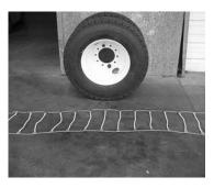
Park vehicle on firm level ground, away from traffic. Unroll the set and lay each half pair on the ground next to the tire it is intended to cover. Make sure that there are no twists or kinks in the cable chain.
