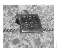
Make sure that the smooth side of the eyelets (marked "TIRE SIDE") are against the tire. If the smooth side is not toward the tire, damage will occur.
