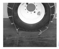
Drape the cable chain over the top of the tire so that both ends can touch the ground and the long metal latch is on the outside of the tire (toward you) and is draped toward the back of the vehicle. Note that the two half sets are made so that one fits on a tire only on the left and one only on the right.
