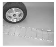
Park vehicle on firm level ground and turn off the engine. On front wheel drive cars, turn the steering wheel for easier access of the inside connection. Chains should be mounted on the "drive tires". Unroll the chain on the ground next to the tire. Position the cable so the end hooks are toward the front of the vehicle.
