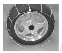
Drape cable chain over the tire so that the smooth side of the cross member hook is against the tire. The cross member nearest the end hook should touch the ground.
