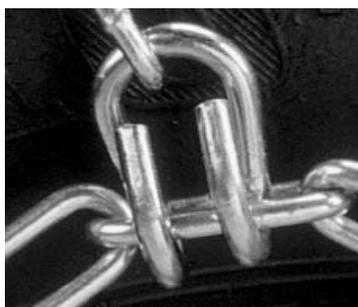
5 The curved portion of the cross chain hooks should face away from the tire.
