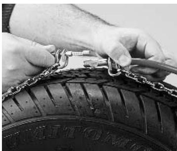
2 Reach around with both hands and grasp the ends of the coated side cable. Pull both ends to the top of the tire and fasten the inside hook. Be careful to avoid twists in any part of the chain.
