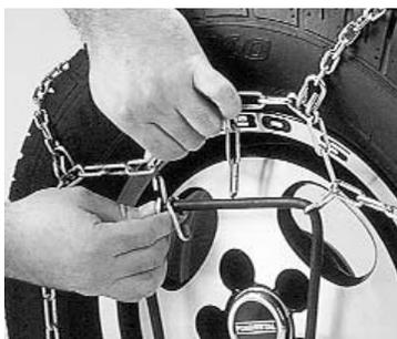
4 Attach the rubber tensioner to equal segments of the side chain, as shown. Make the first connection at about the 5 o'clock position, then at 11 o'clock and so on. Hook any excess side chain with a rubber tensioner hook or wire tie.
