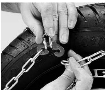
3 Hook the red end fastener on the outside side chain to a corresponding link of the side chain at the top of the tire. Then hook the silver end fastener to the side chain at the bottom of the tire.
