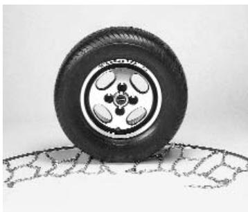
1 Park the vehicle on solid level ground. Set the emergency brake. Lay the chain on the ground with the smooth side of the hooks face up. The split side chain should be positioned closest to you around the bottom of the tire.
