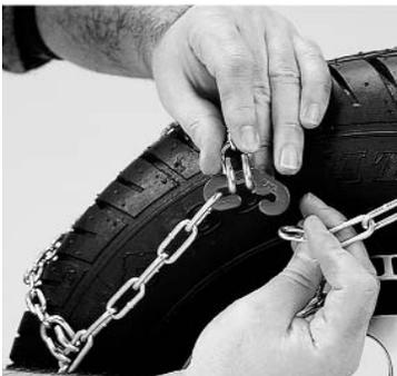
Drive the vehicle off the highway to safe level ground. Turn off the engine and set the emergency brake. The wheel should be positioned so that the red plastic marker is not at the 12 o'clock position on the tire.
