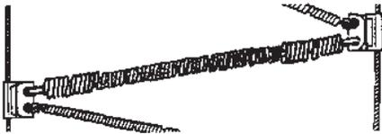
Typical cross member with 3 traction coils on each side free of wear and abrasion. Traction coils are still round and can rotate. All other coils made contact with the road indicating normal use and wear
