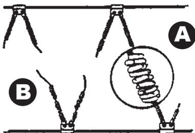
[A] Fragmented traction coils - Traction coils in middle of cross members begin to fragment due to speeds over 30 mph and/or excessive bare pavement driving.
