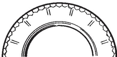
Tire sidewall damage can result from driving at speeds above 30 mph. Chain becomes stationary on the tire and is not permitted to slowly rotate. Another cause could be installing the chain upside down; the metal tabs will dig into the tire.
