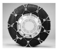
Use at least two rubber tensioners per chain and make sure that the tensioners are seated in all hooks. The vehicle may be driven with no further adjustment.
