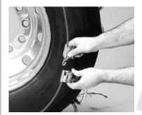
At the inner sidewall, connect the inner end fastener (the "split" in the outside cable can be opened to provide more space for connecting the inside fastener).
