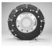
Park vehicle on firm level ground, away from traffic and turn off the engine. Drape chain over the tire. Make sure that the smooth side (TIRE SIDE) of the cross member hooks is against the tire sidewall. The tightener hooks on the side cable must be on the outside of the tire (the side towards you).
