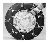
Install the rubber tensioner, always stretching the tensioner from one hook to the one farthest from it (use the included lever tool to make this installation easier).
