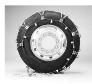
Roll onto the chain by moving the vehicle two or three feet (60-100 cm). Which is the equivalent to 1/4 of a tire revolution.
