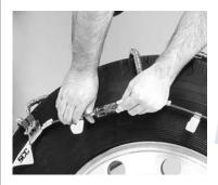
At the top of the outside cable, take the bushing end of the outside split side cable and thread it through the keyhole fastener. Grasp the outside cable with both hands and pull it toward you to create as much slack as possible. Then connect the bottom fastener. See the close-up on the following page for a detailed look at this connection.
