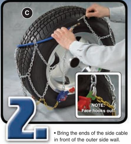
• Connect the side cable together by inserting the knob into the key-hole latch (C) • Leave the connected side cable draped over the outer sidewall (D) while you complete step 3.
