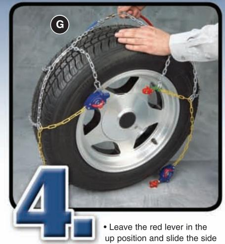
cable to the back of the tire (G), ensure the chain is centered on the tire.
