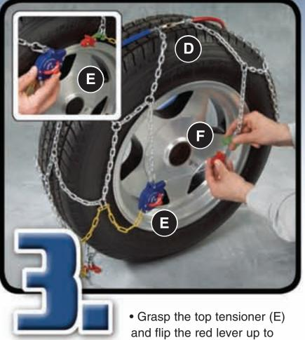
install. Pull the red cable end out and attach to the green side chain connecter (F).
