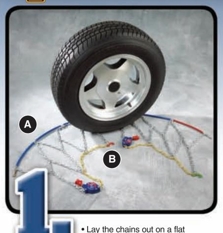
ensure the side wire hooks are facing down. Do not drive with chains that are damaged. • Slide the inside side cable (A) and chain behind the wheel. Find the split (B) in the front side chain. Lay one half of the chain in front of the tire and the other behind the tire.
