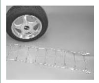
Park vehicle on firm level ground and turn off the engine. On front wheel drive cars, turn the steering wheel for easier access of the inside connection. Chains should be mounted on the "drive tires". Unroll the chain on the ground next to the tire. Position the cable so the end hooks are toward the front of the vehicle.
