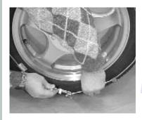
On the outside of the tire, thread the cable with bushings through the end hook for intial mounting. Grasp the outside side cable with both hands and pull it towards you. This will create as much slack as possible. Then make the outside connection in the same manner as the inside.
