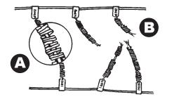
[A] Fragmented traction coils - Traction coils in middle of cross members begin to fragment due to speeds over 30 mph and/or excessive bare pavement driving.
