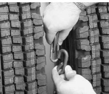
4 Reach behind the tire and engage the inside connector making sure it is as tight as possible. Then connect the center (between the duals) fastener in the same manner. See the illustration on the next page for a detailed look at this connection.
