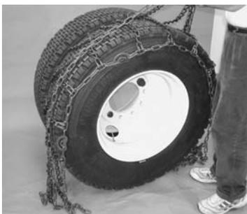
1 Park vehicle on firm level ground, and turn off the engine. Set the parking brake. Lay the chains out flat on the ground, making sure there are no twists or tangles. Make sure the cross chain hooks are facing upward.
