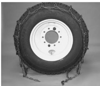
2 Drape the chain over the tire, so that one cross chain is positioned at the point where the tire meets the ground. Again make sure the cross chain hooks are facing upward. Hooks that face down (towards the tire) will cause damage to the tire.
