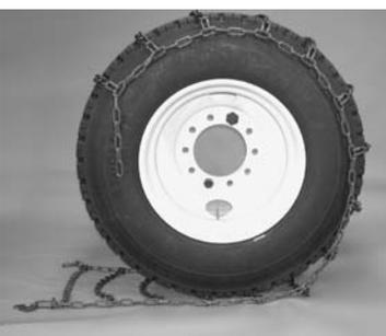
3 Drive forward a few feet, far enough so that one or two of the cross chains pass under the tire.
