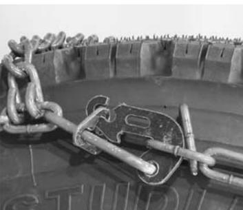
5 Next fasten the outside fastener, again making sure it is as tight as possible. Drive a short distance and retighten all fasteners. For best results, make sure all connections are equal and as tight as possible.
