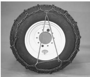
Security Chain Co. recommends that chain tighteners (sometimes known as chain spreaders) be used to take up additional slack. To make this simpler, attach the first hook at the “11 o’clock” position, the next at the “5 o’clock” position and so forth. The open side of the hooks must face away from the tire. No further adjustment should be necessary.
