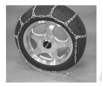
Drive forward a few feet, far enough so that one or two of the cross chains pass under the tire
