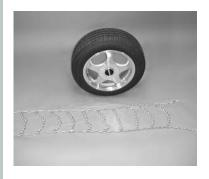
Park vehicle on firm level ground, and turn off the engine. Set the parking brake. Unroll the chains and lay them out flat on the ground making sure there are no twists or tangles. Make sure the smooth side of the cross chain hooks are towards the tire.
