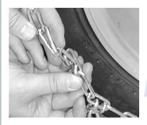
Reach behind the tire and engage the inside connector on the 2nd or 3rd link. See the illustration on the next page for a detailed look at this connection.
