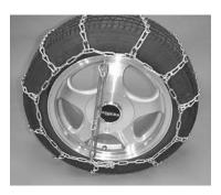
Security Chain Co. recommends that chain tighteners (sometimes known as chain spreaders) be used to take up additional slack. To make this simplier, attach the first hook at the "11 o'clock" position, the next at the "5 o'clock" postion and so forth. The open side of the hooks must face away from the tire. No further adjustment should be necessary.
