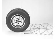
Park vehicle on firm level ground, away from traffic and turn off the engine. Set the emergency brake. Remove any wheel covers. Chains should be installed on drive tires. Lay the cable chain on the ground with the smooth side (TIRE SIDE) of the cross member connection up.
