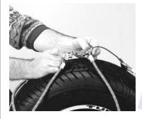
Reach around each side of the tire and grasp both ends of the non-split cable (the cable that is furthest away from you). Pull both ends to the top of the tire so the fasteners can be seen and manipulated more easily. Fasten the curved "C" hook through the fastener hole.
