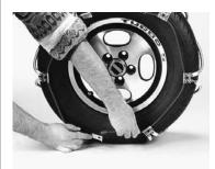
Take the bushing end of the lower fastener and thread it through the lower keyhole (the one near the ground), using the same process as the top fastener. Please refer to the following page for a detailed look at making this connection
