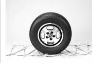
Move the chain in a sweeping motion under the vehicle so the open mid-section is positioned up against the backside of the tire. This sweeping motion can best be done while kneeling in front of the tire.
