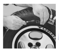
At the top of the outside cable, take the bushing end of the outside split side cable and thread it through the keyhole fastener. Grasp the outside cable with both hands and pull it toward you to create as much slack as possible.
