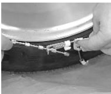
At the inner sidewall, make the connection on the inside of the tire by pushing the cable with end bushings behind the tire and toward the front of the vehicle.
