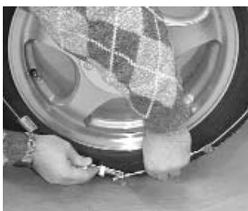
On the outside of the tire, thread the cable with bushings through the end hook for initial mounting. Grasp the outside side cable with both hands and pull it towards you. This will create as much slack as possible. Then make the outside connection in the same manner as the inside.
