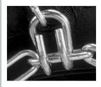
The curved portion of the cross chain hooks should face away from the tire.
