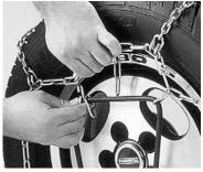
Disengage the rubber tightener and unhook the outside side chain, then the inside hook fastener. Reach behind the tire and pull the hoop apart and off of the tire, so that it is laying flat on the ground. Then drive off the chain.
