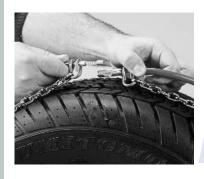
Reach around with both hands and grasp the ends of the coated side cable. Pull both ends to the top of the tire and fasten the inside hook. Be careful to avoid twists in any part of the chain.
