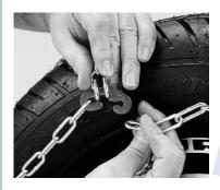
Hook the red end fastener on the outside side chain to a corresponding link of the side chain at the top of the tire. Then hook the silver end fastener to the side chain at the bottom of the tire.
