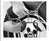
Attach the rubber tensioner to equal segments of the side chain, as shown. Make the first connection at about the 5 o'clock position, then at 11 o'clock and so on. Hook any excess side chain with a rubber tensioner hook or wire tie.
