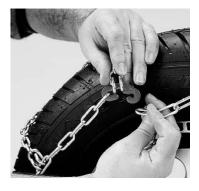
Drive the vehicle off the highway to safe level ground. Turn off the engine and set the emergency brake. The wheel should be positioned so that the red plastic marker is <u>not</u> at the 12 o'clock position on the tire.
