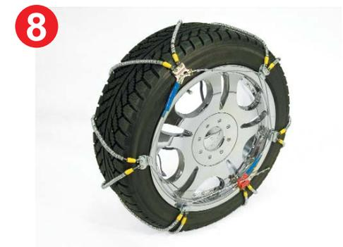
8 This is how a properly installed chain should appear on your tire. Your vehicle may now be driven without further adjustment.
