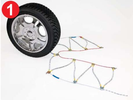
1 Park vehicle on firm, level ground and away from the flow of traffic. Set the emergency brake. Chains should be installed on drive wheels. Lay the cable chain on the ground with smooth side (TIRE SIDE) of the crossmember hooks up.
