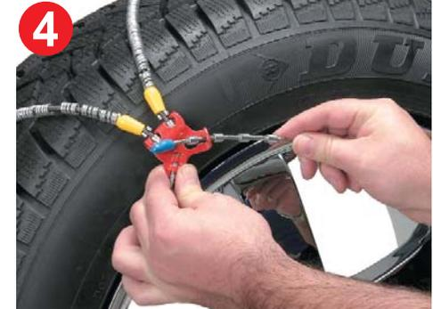
4 Grasp the outside cable with both hands and pull it toward you to create as much slack as possible. Connect the top fastener (the red one) as tightly as possible by inserting the silver "beads" on the cable through the keyhole.
