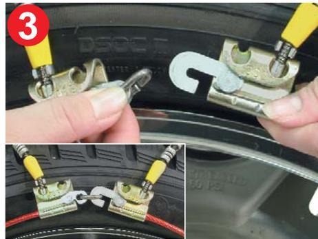
3 Reach around each side of the tire and grasp both ends of the non-split side cable (that is furthest away from you). Pull both ends to the top of the tire so the fasteners can be seen and manipulated more easily. Connect the inside fastener.
