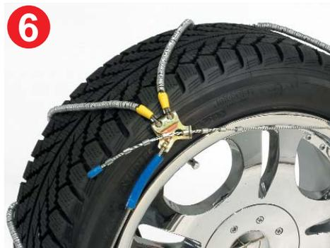
6 Move the vehicle a few feet. Remove cable "slack" by retightening both adjustment points as equally as possible.
