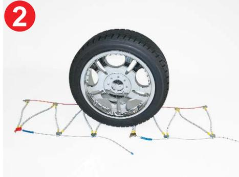
2 Move the chain in a sweeping motion under the vehicle so the open mid-section is positioned up against the backside of the tire. This sweeping motion can best be done while kneeling in front of the tire.
