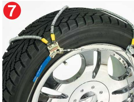
7 To secure the free ends of the cable, slide the plastic spirals over them with a twisting motion. If insufficient cable is available for plastic spirals to secure, "tuck" the short end up next to the crossmember anchor points, as shown here.
