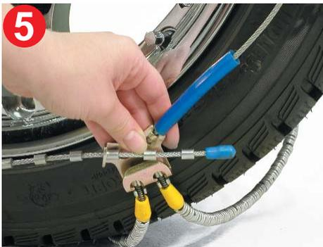
5 Repeat this process with the gold adjustment fastener. Ensure that both fasteners are adjusted within one bead of each other.
