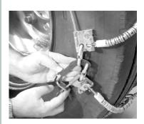
Connect the outside latch fastener and secure with link.
