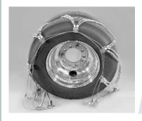
Keep the cable chain folded and drape it over the top of the outside tire. Both sidecables are at the front of the tire.
