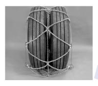
Flip top half of the chain over the top of the inside tire. Make sure that the smooth sides of the eyelets (marked "TIRE SIDE") are against the tire.
