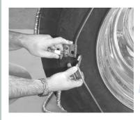
Roll 1/4 of a tire revolution onto the chain. Connect the inside speed hook.
