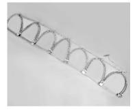
Park the vehicle in a safe area on level ground and set the emergency brake. Lay the chains out on the ground next to the tires they are intended to cover. Fold chain in half lengthwise. Both sidecables should be in front of you. The sidecable with the black fastener should be on the ground.
