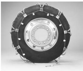
Park vehicle on firm level ground, away from traffic and turn off the engine. Drape chain over the tire. Make sure that the smooth side (TIRE SIDE) of the cross member hooks is against the tire sidewall. The tightener hooks on the side cable must be on the outside of the tire (the side towards you).
