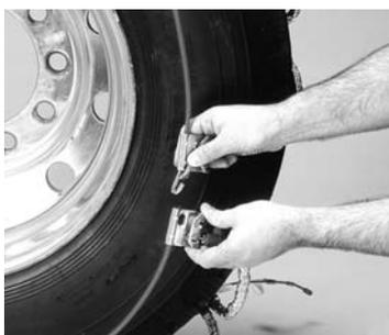
At the inner sidewall, connect the inner end fastener (the "split" in the outside cable can be opened to provide more space for connecting the inside fastener).
