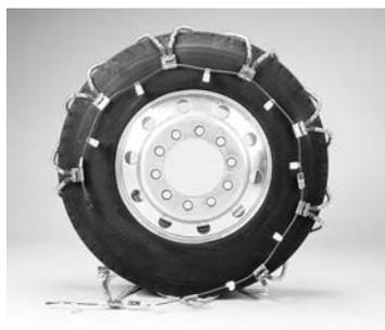
Roll onto the chain by moving the vehicle two or three feet (60-100 cm). Which is the equivalent to 1/4 of a tire revolution.
