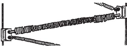
Typical cross member with 3 traction coils on each side free of wear and abrasion. Traction coils are still round and can rotate. All other coils made contact with the road indicating normal use and wear
