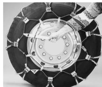
Install the rubber tensioner, always stretching the tensioner from one hook to the one farthest from it (use the included lever tool to make this installation easier).
