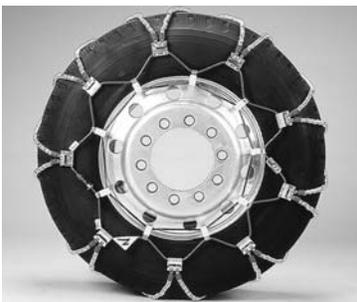
6 Use at least two rubber tensioners per chain and make sure that the tensioners are seated in all hooks. The vehicle may be driven with no further adjustment.
